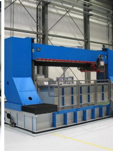
**Friction Stir Welding (FSW)**
