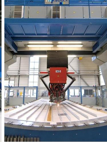
**Laser Beam Welding (LBW)**
